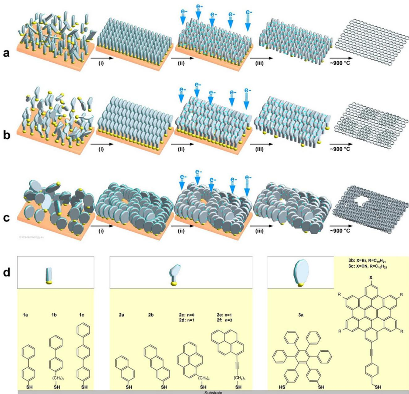
Fig. 1: Schematic for the formation of carbon nanomembranes (CNMs) and graphene from molecular precursors. (a-c) Schematic illustration of the fabrication route for CNMs and graphene; (d) Chemical structures of the different precursor molecules used in this study.
